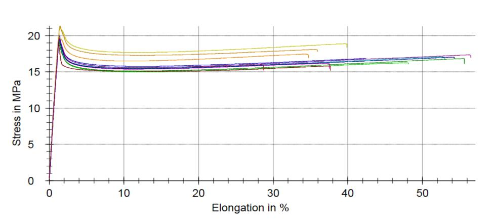
The impact resistance and tensile strength tests show that the composites in which pseudoboehmite treated with octadecylamine were used showed higher values than the composites containing only pseudoboehmite and HIPS
